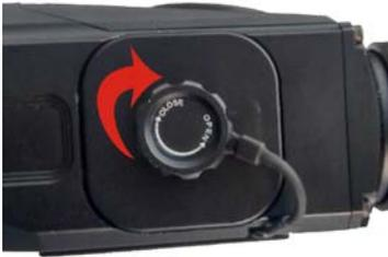
Fig.8 close batteries cover
