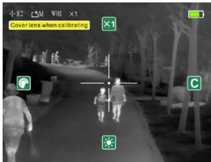
Fig. 21 the background calibration interface
